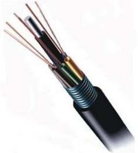
The loose tube stranding technology make the fibers have good secondary excess length and allow the fibers free movement in the tube, which keeps the fiber stress-free while the cable is subjected to longitudinal stress.
